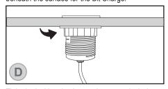
Tight the locking ring by turn it counterclockwise until it is tighten strongly to the surface and verify the Innera Bit Charge is firmed and cannot be rotated.
